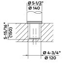
Cast-in in finished floor level
